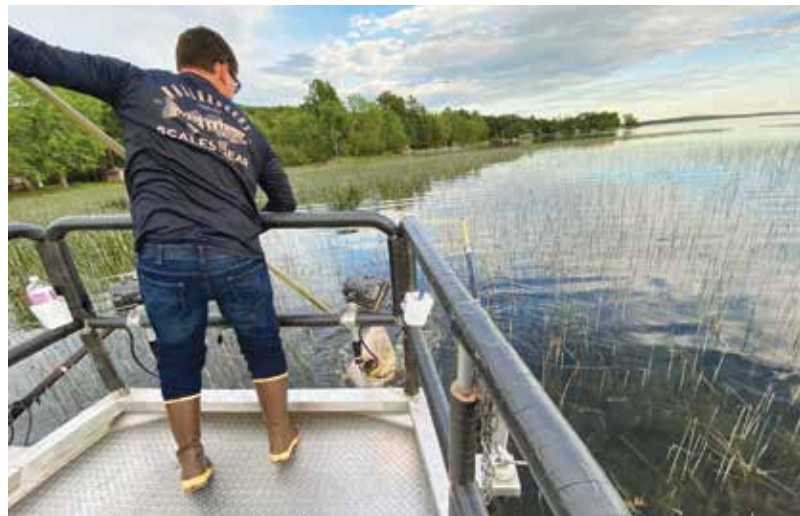
(Above) Mole Lake Fisheries staff member Norb Nunway harvests adult bullheads aboard one of Mole Lake Fisheries electroshocking watercraft. As the boat coasts slowly through the emerging bulrushes, electrodes dangling in the water momentarily paralyze the fish, allowing just a second or two to selectively net only bullheads, as many as possible, before they come to and scurry away — and before the net gets too heavy to hoist on board and deposit into the live well. Driving the boat is Mole Lake Fisheries staff member, Clint Soulier (not pictured).
